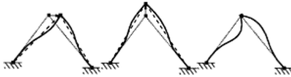
FIGURE 6.6 Compatibility between nodal and element end displacements.
